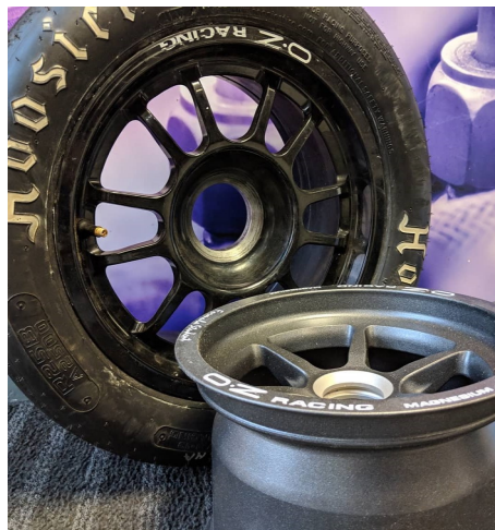
Comparison of old 13-inch wheels and new 10-inch wheels
