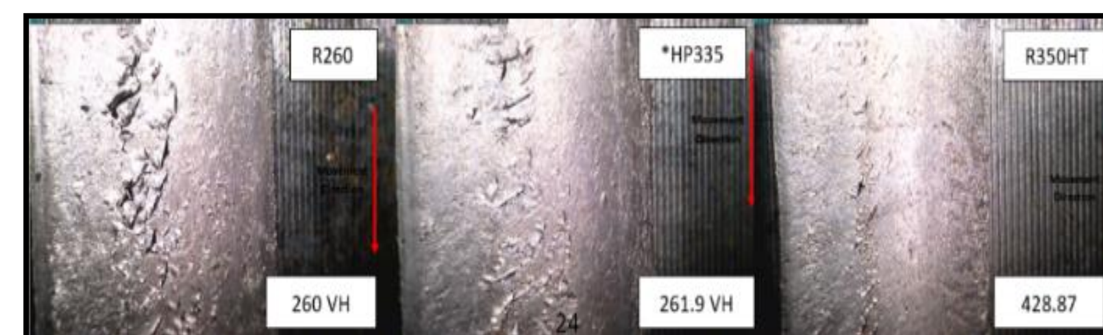
Figure 3- An annotated photograph of RCF cracks on tested samples
